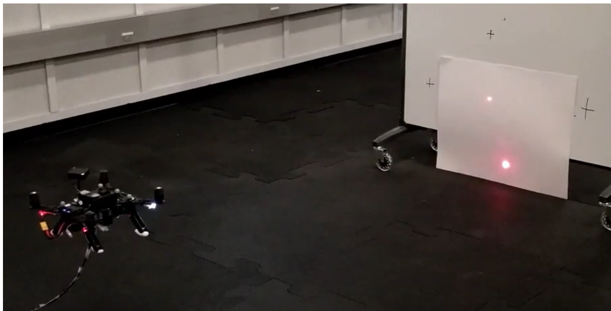
(a) Our UAV setup with Intel Aero UAV and our LiDAR mounted on it.
