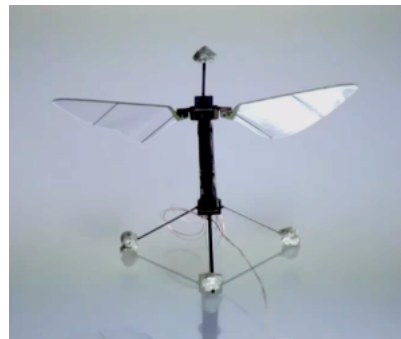
Fig. 1. An Image of the RoboBee as developed at the Harvard Micro-Robotics Lab
